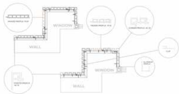
SHORT DIAGRAM OF VERTICAL INSTALLATION OF FACADE BOARDS
